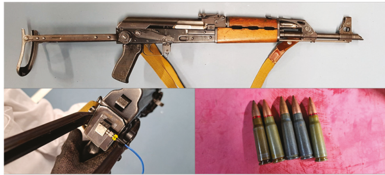
Figure 1. Measurement of vibrations emitted by a Zastava M70 AB2 automatic assault rifle. Top: rifle overview; bottom left: accelerometer positioning; bottom right: 7.62 × 39 mm M43 rounds.
