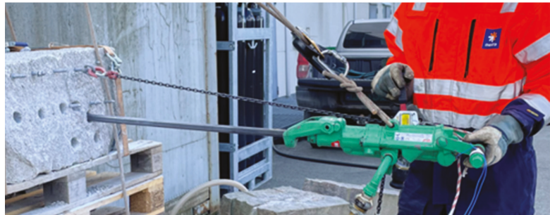
Figure 1. Laboratory setup to recreate drilling conditions with current equipment when operators are horizontally drilling for the insertion of rock bolts. Prior to drilling the main hole, a smaller (8–10 mm), expanding bolt with an eye nut is placed to anchor the hoist chain. A lever hoist is used to control the feed force during drilling.
