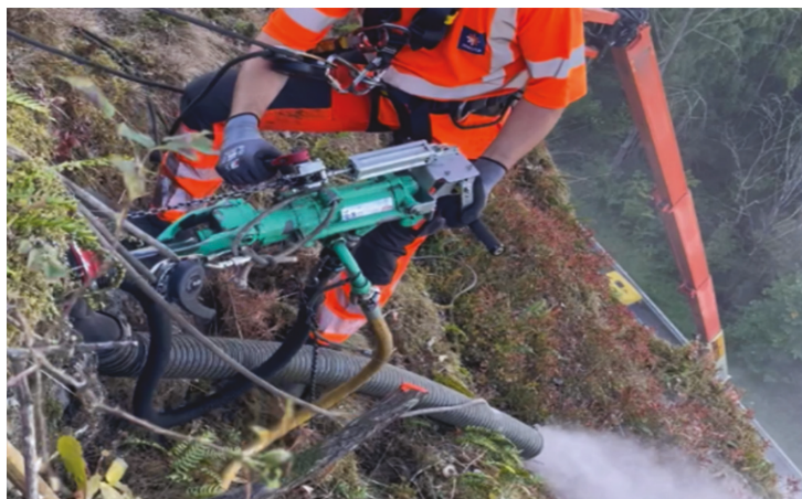
Figure 4. The prototype without ATVA being tested in the field in Norway with the dust removal device.
