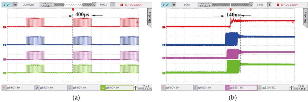
**Figure 15.** System device control synchronization test result diagram: (a) pulse output waveform of each slave under a 200 μs time scale; (b) pulse output waveform of each slave under a 80 ns time scale.
