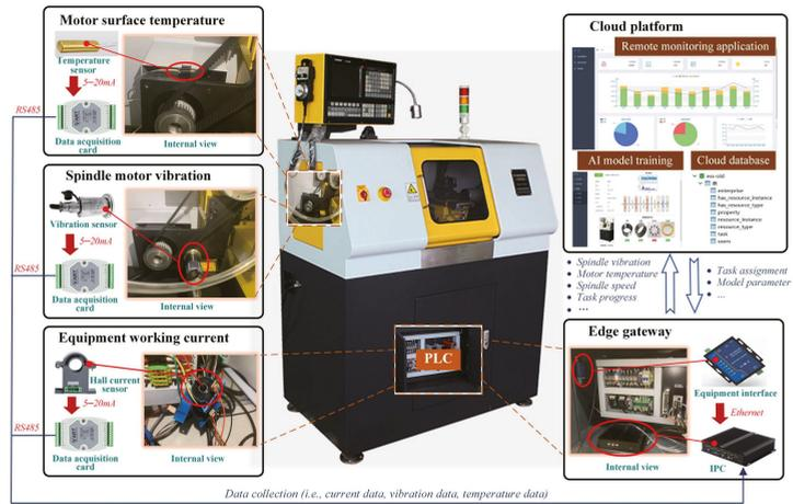
Figure 6. Digital transformation of the CNC lathe.
