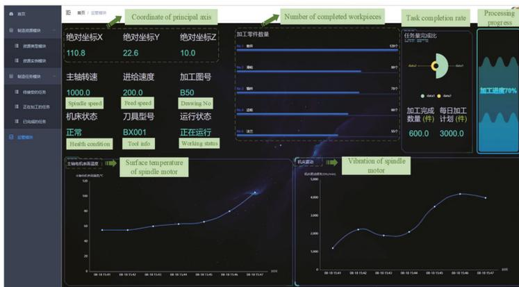
Figure 8. Remote monitoring of equipment working status.
