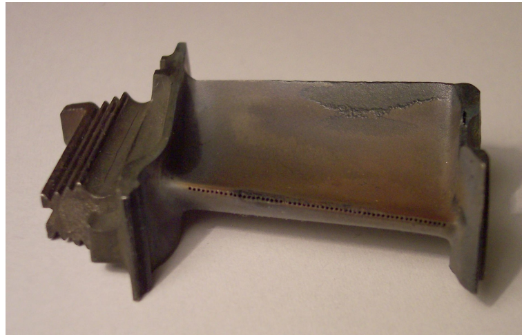
Figure 3. Damaged blades resulting from exposure to high temperature and stress [17].
