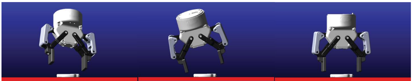
Figure 3. Model of robotic gripper and the object to be gripped in ADAMS/View with different rotation settings. Source: Own.
