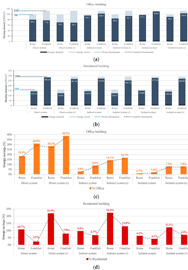
Figure 9. Heating energy demand in winter season: (a) office building; (b) apartment building; (c) percentage of energy saving in office building; (d) percentage of energy saving in residential building.
