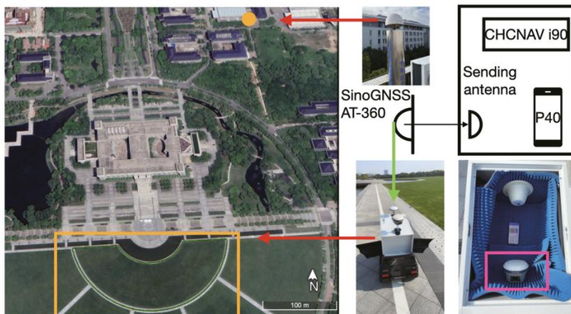
Figure 10. Layout of the smartphone and receiver for collecting kinematic datasets.
