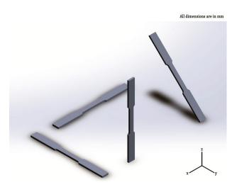
**Figure 1.** Dog-bone shaped specimens built in four different configurations in SLM building platform and their dimensions.
