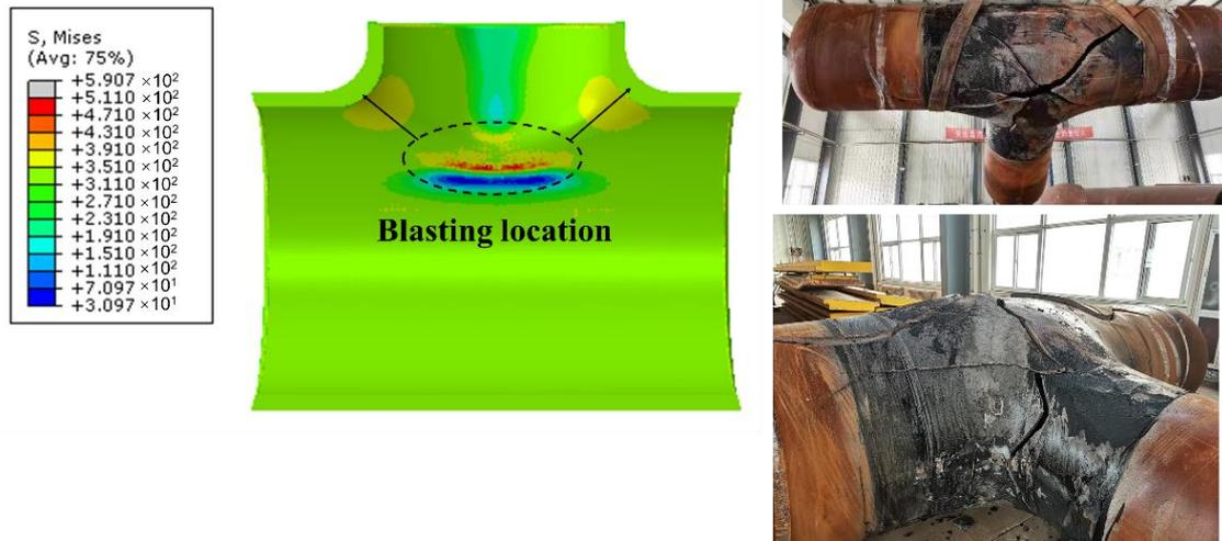
**Figure 21.** Simulated prediction and experimental verification of the blasting location for the SSESS repaired low-strength tee.
