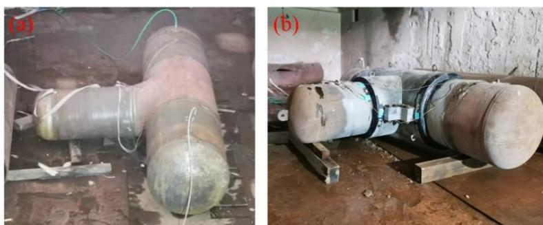
**Figure 11.** Hydraulic test structural part: (a) unrepaired tee, and (b) SCESS repaired tee.
