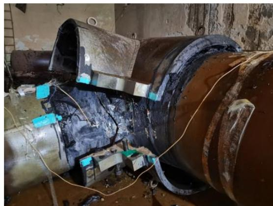
Figure 19. Failure of SCESS with bolt fracture.
