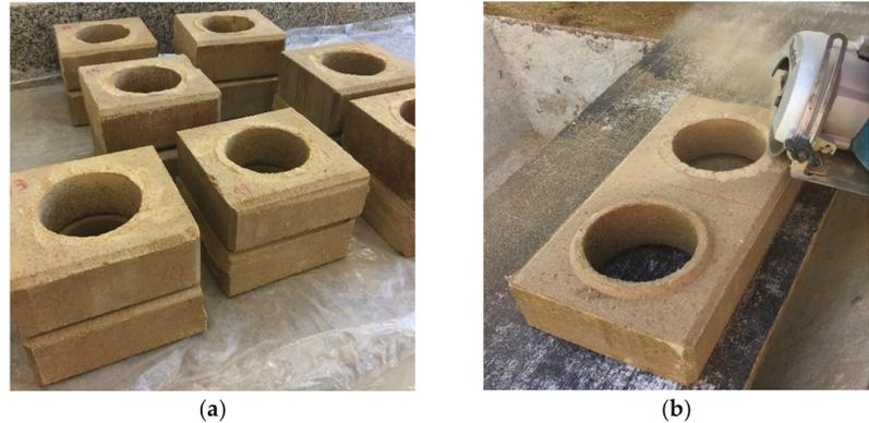
**Figure 2.** Brick capping step: (a) Bricks cut in half; (b) upper part of socket removed.
