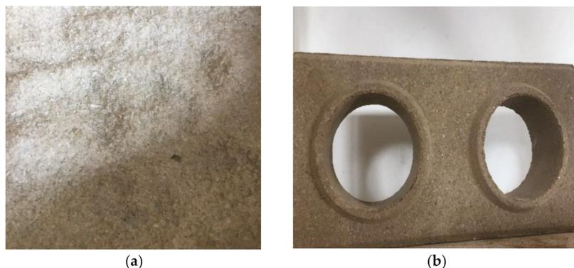
**Figure 1.** Materials used: (a) PET waste; (b) soil-cement brick.
