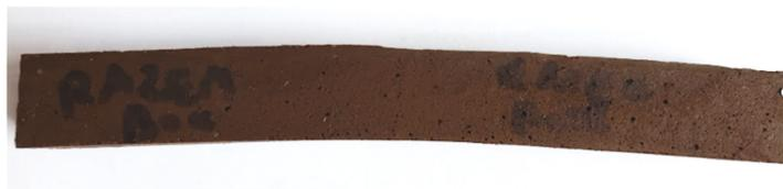
**Figure 10.** The view of pores of glass wool-based geopolymer mortar with bauxite.
