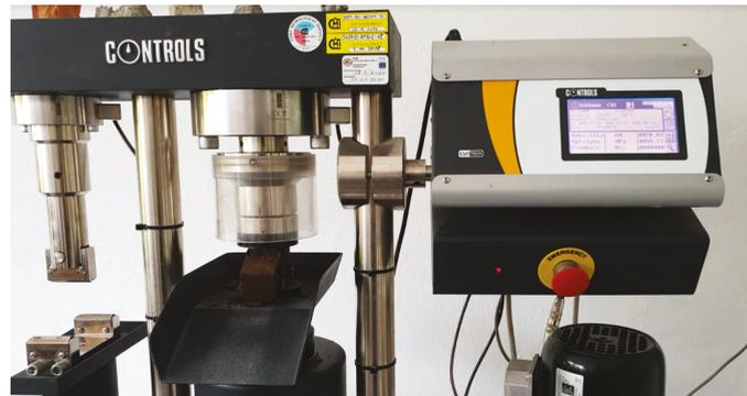
Figure 6. The view of the sample of geopolymer mortar under testing of the compressive strength.
