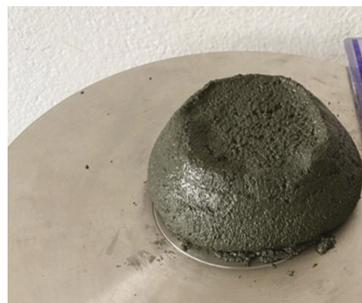
Figure 8. The view of slump-flow of glass wool-based geopolymer fresh mortar with  $Al_2O_3$ .
