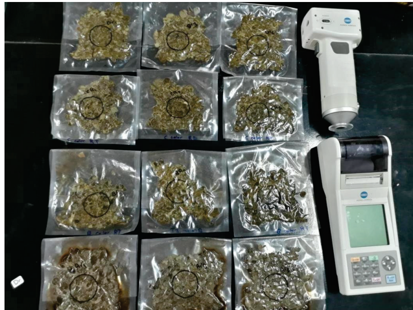
Figure 1. Oregano mix as the finished product was prepared for color index ( L^*a^*b^* ) measurement.
