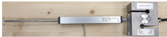
Figure 3. Strain gauge sensor (on the left); force gauge sensor (on the right).
