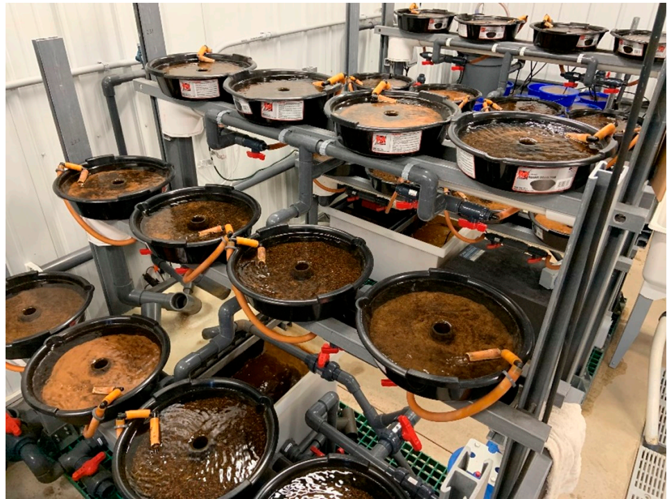
Figure 6. The Minnesota Zoo’s native mussel facility includes individual rearing pans which allow for manipulation of metrics such as substrate, flow rate, and mussel density to facilitate experimentation. Water is circulated from a nearby lake.
