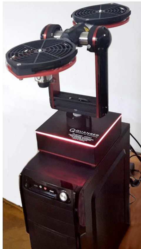
Figure 1. Quanser Aero 2 laboratory equipment with a 1-DOF configuration.
