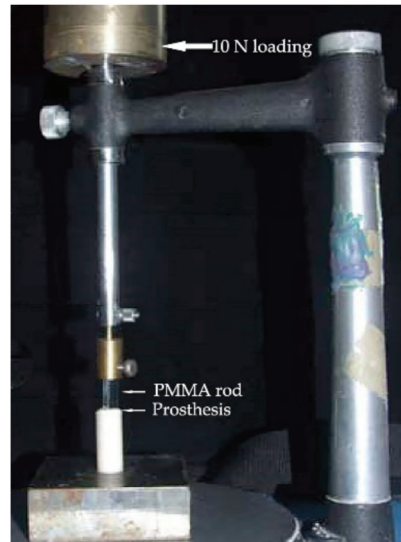
Figure 1. A prosthesis bonded to PMMA rod vertically aligned and loaded using a surveyor.
