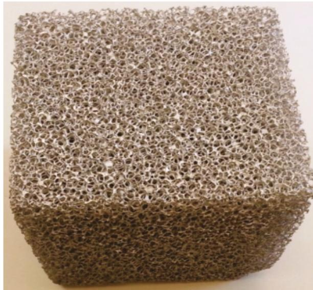
**Figure 1.** Photograph of a block of open-cell aluminum foam with 20 pores per inch. (Photo taken by author).
