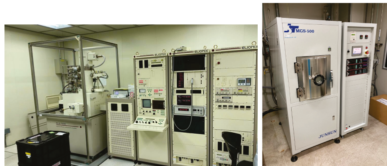
Figure 18. Electron beam lithography machine located in (Left) Academic Sinica laboratories (EBL, ELS-7000 ELIONIX); and (Right) Junsun Tech MGS-500 sputtering machine installed at the NEMS center of NTU.
