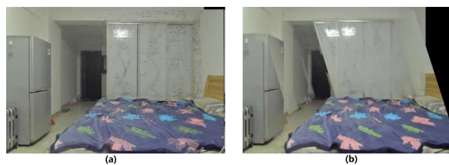
Figure 21. Image stitching experiment. (a) Image stitching effect based on depth information layering; (b) Image stitching effect based on ORB feature points.
