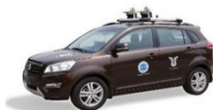
Figure 1. Unmanned vehicle with two 32-line lidars.
