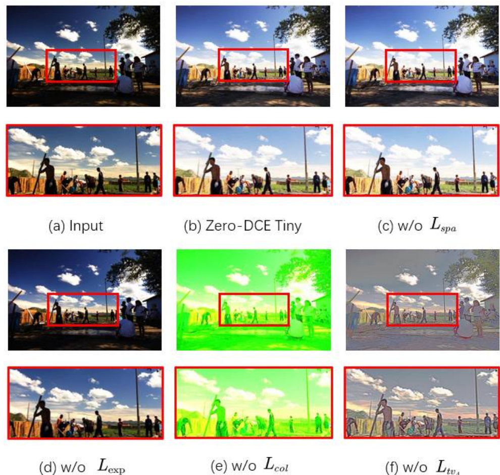
Figure 5. Ablation study of each loss. Subfigure (a) shows the original input, subfigure (b) shows the enhanced image result through Zero-DCE Tiny method, subfigure (c–f) respectively show the image enhancement results after removing spatial consistency loss, exposure control loss, color consistency loss and illumination smoothness loss.
