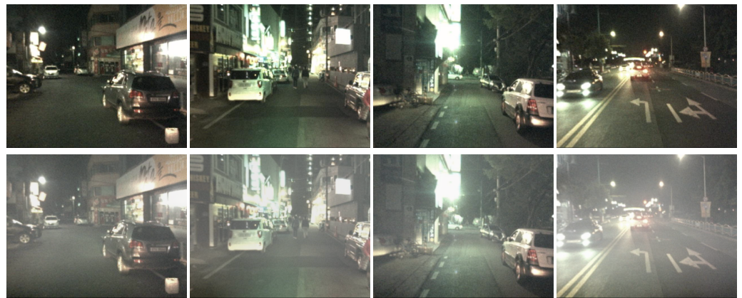
Figure 4. The proposed method for synthesizing nighttime hazy images. The first row shows original clear night scenes from [39], and the second row shows the synthesizing hazy images.
