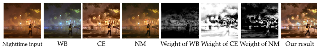
Figure 1. We exploit a multi-scale gated fusion network for nighttime haze removal. The first column gives degraded inputs. The second, third, and fourth columns show derived inputs for original images. The learned confidence maps for the derived inputs are shown in the fifth, sixth, and seventh columns, respectively. The last column shows our results by the proposed algorithm.
