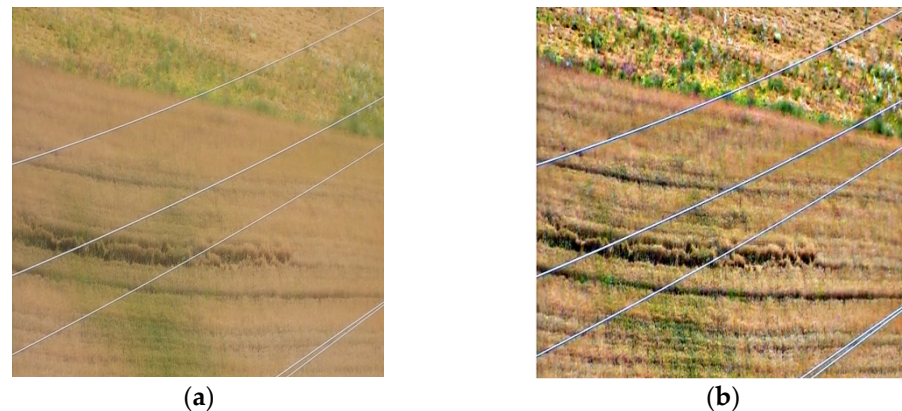
Figure 1. Power line scene image enhancement by using a guided filter. The input image itself is selected as the guided image. (a) Power line image. (b) Enhanced image.
