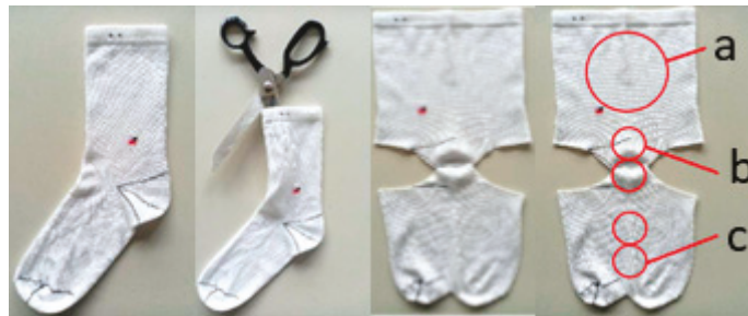
Figure 5. Cutting the socks and the sampling of the test specimens: (a) for testing the propensity to surface pilling, mass per unit area and water vapor absorption; (b,c) for testing the abrasion resistance.
