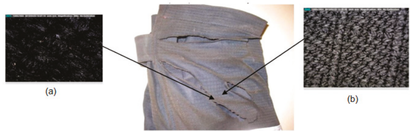
Figure 9. Damage to the sleeve of the overalls made with a Dino-Lite microscope in two different magnification: (a) 184 \times ; (b) 60 \times .
