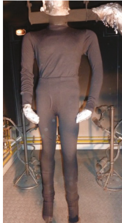
Figure 1. Tested underwear on the fire manikin.
