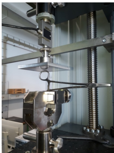
Figure 2. Experimental array for determination of the force (N) required to lock the jaws of the needle holder using the clamp mechanism. It was found to be 35 N.
