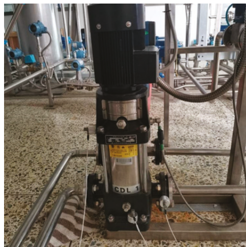
Figure 12. Layout of measuring points of centrifugal pump.
