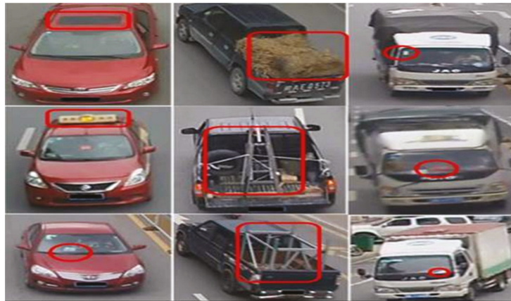
Figure 11. Shows vehicles that are same in global appearance but differentiated by local regions that are marked in red circle.
