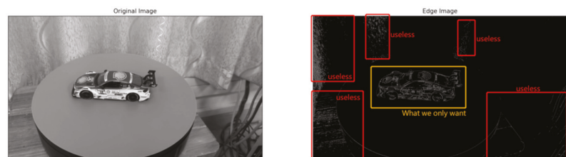
Figure 1. The matting result of the Canny algorithm.
