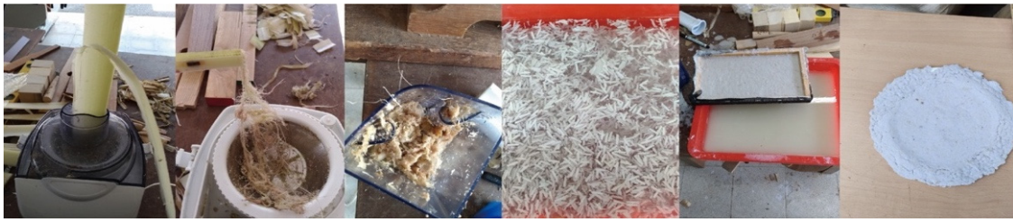
Figure 16. Evolution of the material-tinkering experiment conducted using shredded materials mixed with pulp and the prototype of design concept by craftsman Jing-Teng Lin (left to right: shredding, fibre extraction, reduction in fibre length, mixing with pulp, papermaking using banana fibre mixed with pulp, and papermaking mould for banana fibre mixed with pulp). (photographed by 1st author).
