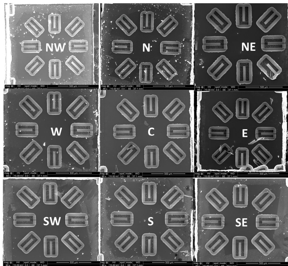
Figure 7. Top view SEM images of cantilevers formed from a 5-layer, 500 nm total thickness, PVD deposited Al 0.68 Sc 0.32 N where the process gas flow for each layer is linearly changed from 30 to 20 sccm
