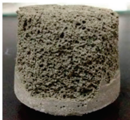
Figure 11. The pores in backfilling body.
