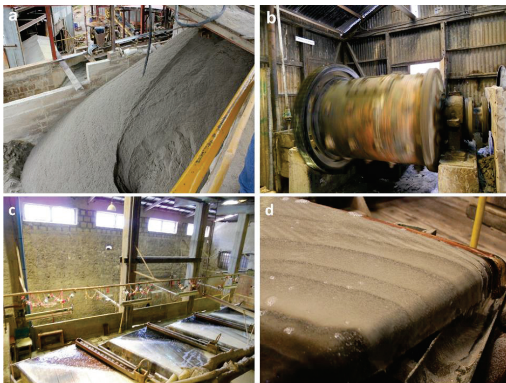
Figure 3. View of the Catavi processing plant: (a) feed tailings; (b) ball mill for the comminution; (c), view of one of the three floors with the material being processed in the shaking tables; (d), detail of the gravity separation in a shaking table.
