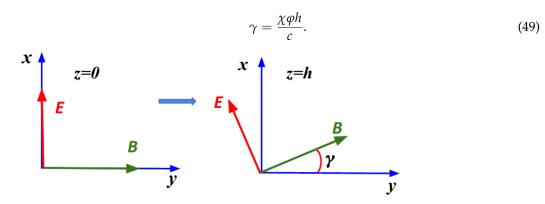
Figure 1. Faraday effect of polarization rotation under the action of uniform axial torsion.
