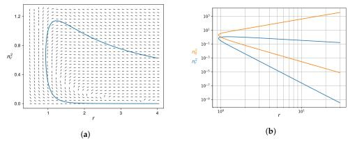
**Figure 2.** Solution for the torsion field with cylindrical symmetry with  $n_r \neq 0$ , k = 0, and  $k_{\theta} = 1$ . (a) The flow field when k = 0 and  $k_{\theta} = 1$  and the particular solution satisfying  $n_r^2 = 1$  when r = 1. (b) The same solution for  $n_r^2$  on a log–log plot and the accompanying function  $n_{\theta}^2 = 1/(r^4 n_r^2)$ .
