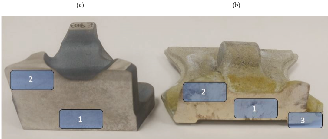
Figure 8. Microstructure test areas, (a) preform, (b) forging.
