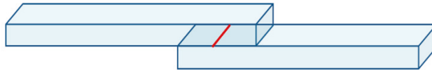
Figure A1. The two bars in contact before deformation. The red line indicates the path at the center of the contact area, along which the mechanical fields were extracted.
