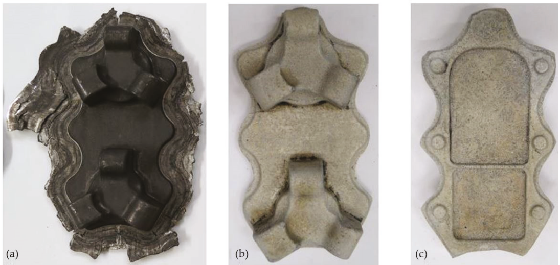
Figure 14. Forging obtained for a preform with a lower degree of forging (variant I): (a) after forging, (b) top view after trimming, (c) bottom view after trimming.
