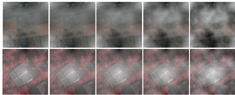
Figure 6. Illustrations of five severity levels of fog rendered the ISPRS dataset. First row: Potsdam. Second row: Vaihingen
