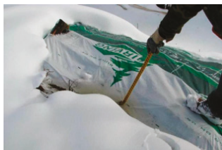
Figure 5. Plastic-based tarps after six months.
