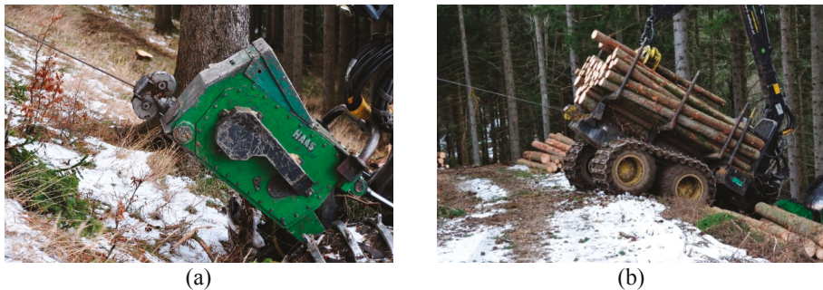
Figure 1. Observed John Deere 1170 E harvester with a mounted winch in the front (a) and a John Deere 1110 E forwarder with an integrated winch (b).
