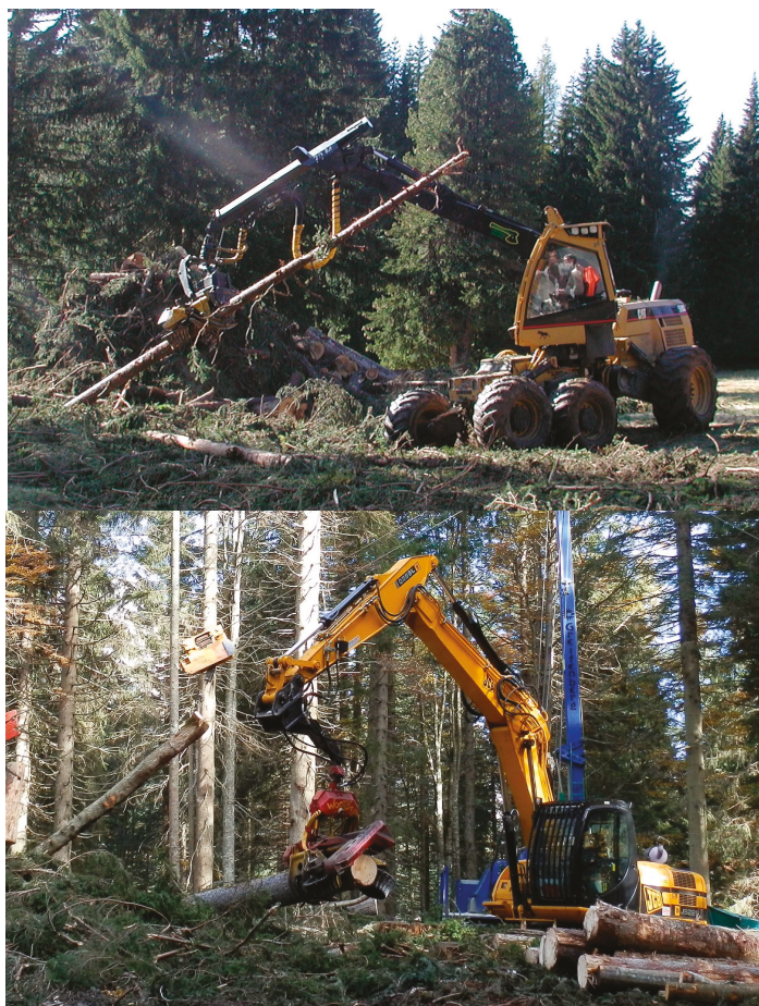
Figure 1. Example of the purpose-built ( top ) and excavator-based ( bottom ) units in the study. These are respectively unit # 2 and # 6.
