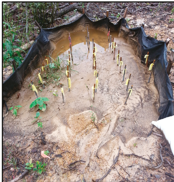
Figure 4. An example of the silt fence sediment traps used in the study. Sediment pins were driven into trap area on a grid pattern and measured at regular intervals.
