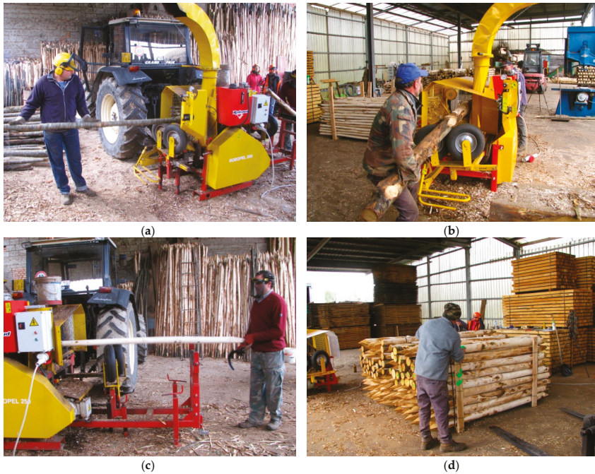
Figure 1. Typical postures assumed during post debarking at the two main work stations: loading-push (a), loading-hold (b), unloading-pull (c), and unloading-stack (d).
