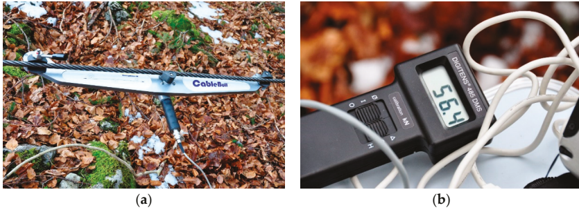
Figure 3. The CableBull cable tensile force measurement device from the German manufacturer Honigmann based on the clamped-on tension monitoring system (a) and the handheld device for checking tensile forces (b).
