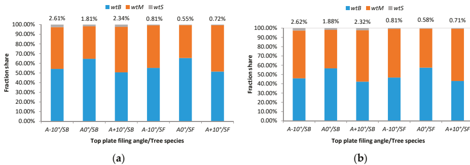
Figure 2. Dependency of sawdust weight structure on top plate filing angle ( A ) and tree species ( S ): (a) chain producer 1 and (b) chain producer 2. Note: wtB —big particles (more than 3 mm), wtM —medium-sized particles (3–0.125 mm) and wtS —small (inhalable) particles (less than 0.125 mm).
