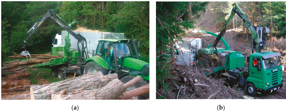
Figure 1. Example of a tractor-powered—or PTO-driven (a) and an independent-engine chipper (b).
