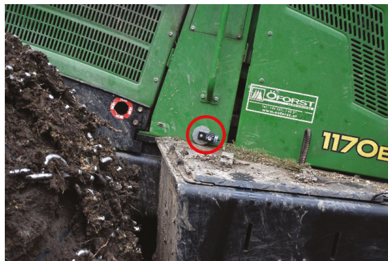
Figure 4. The location of the mounted acceleration data logger on the rear frame of the machinery.
