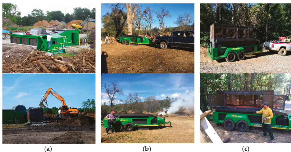
Figure 1. The Air Curtain Burners used to test burning of forest residues in (a) S-220 in Jacksonville, Florida; (b) BurnBoss in Groveland, California; and (c) BurnBoss installed with ember screen in Volcano, California. The loader is used to load the forest residues in S-220 operation while BurnBoss operation is loaded by hand.
