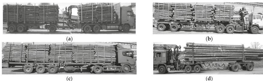
Figure 2. Examples of truck units: (a) truck and trailer, (b) truck and semi-trailer, (c) truck and lightweight platform semi-trailer and (d) truck and dolly.
