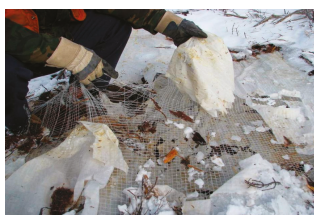
Figure 6. Paper-based tarp after six months.
