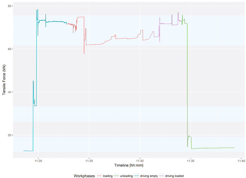
Figure 12. Tensile force graph showing one cycle of the observed forwarder over time with the assigned working phases.
