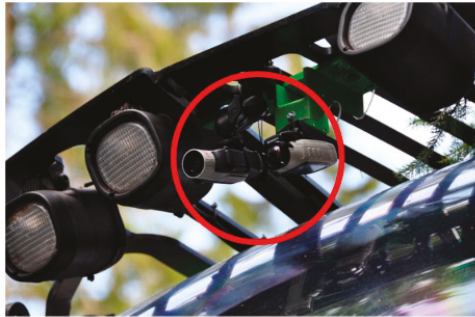
Figure 5. Installed video capturing technology at the protective grating above the front windscreen for recording harvesting activities. The second camera ensured data recording in case of failures.
