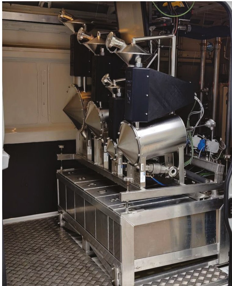
Figure 6. Standard measuring vessels used in the new generation of the AMSV system.
