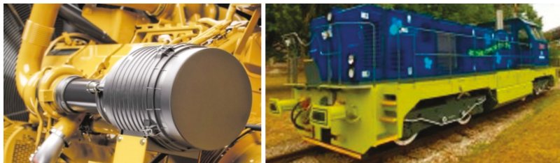
Figure 8. CNG engine and its application in an experimental rail vehicle.
