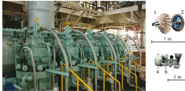
Figure 1. Engine 5S60MC and TCA 66-20072 turbocharger, 1—compressor wheel, 2—turbine rotor, (a,b)—acoustic measuring points.
