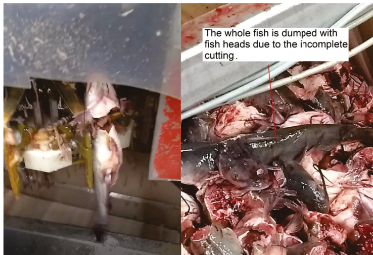
Figure 6. The waste due to deheading processes.
