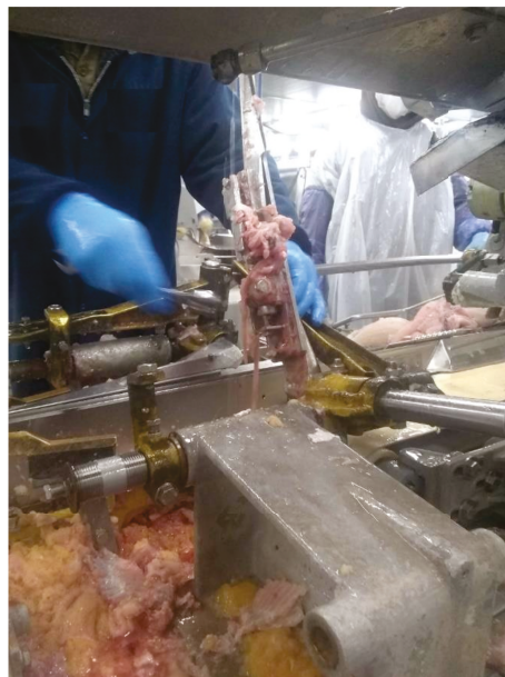
Figure 4. The manual cleaning process for the filleting machine.
