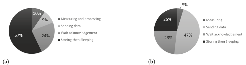
Figure 9. Time distribution between the different steps in the worst-case scenario, for two use cases. (a) Use case I; (b) Use case II.
