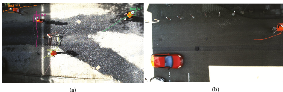
Figure 9. Examples of the classical tracking system applied to different scenes. (a) An example of the tracking system applied to Scene 2 shows that the tracking is sufficient even on slightly overexposed scenes. (b) On Scene 3, the tracking results show that the worker is tracked successfully while the moving vehicle remains untracked as intended.
