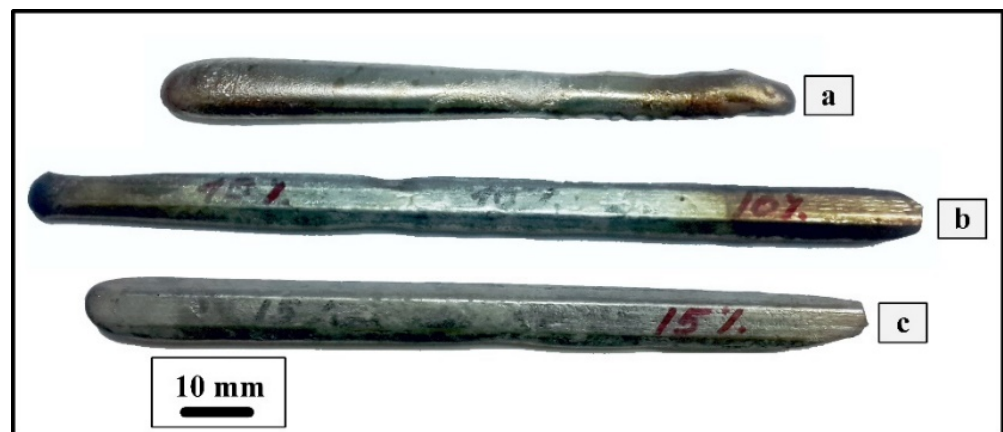
Figure 1. Images of TiNiHf initial ingots obtained by electron beam melting in a copper water-cooled stream-type mold: 1.5 at.% of Hf (a), 3.0 at.% of Hf (b), and 5.0 at.% of Hf (c).
