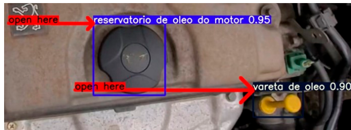
Figure 3. Example of object detection on a test image, where the engine oil reservoir and oil dipstick are detected.
