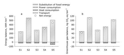
**Figure 2.** The energy (**a**) and GHG (**b**) balances of the energy production at model plants with heat exchangers installed. Scenarios were (S1) slurry and deep litter; (S2) slurry and straw; (S3) slurry, deep litter, and maize silage; (S4) slurry, deep litter, and organic waste; and (S5) slurry, deep litter, organic waste, and organic grass–clover.
