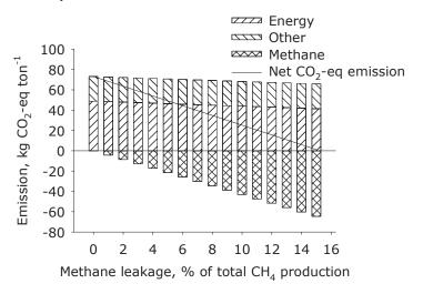
Figure 8. Effect of methane leakage on the climate impact for model plant (S1) with 45 days HRT. Methane and nitrous oxide emissions shown are from storage of livestock manure and biogas slurry.
