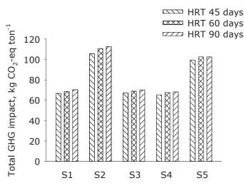
Figure 7. Effect of hydraulic retention time in AD reactor on total GHG impact.
