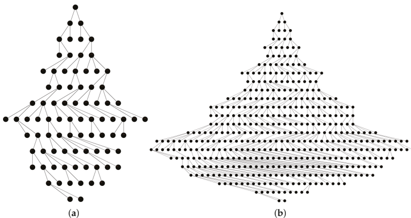
Figure 4. The impact of the Algorithm 2 on graph. (a) The graph without cycles, m = 0 , \bar{n} = n = 83 ; (b) the graph with m = 2 ( \bar{n} = 443 ).
