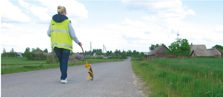
Figure 2. Measurement of crack length with a distance wheel.
