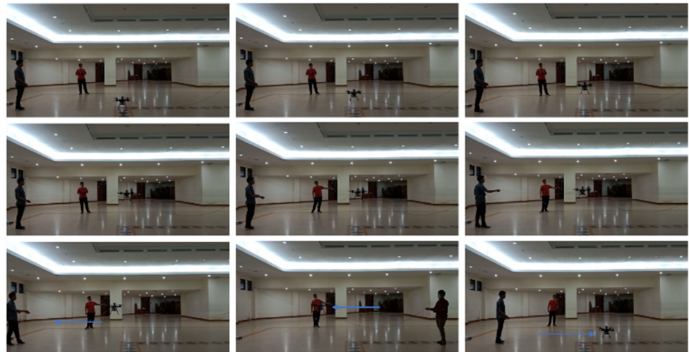
Figure 10. Adding disturbance by pulling the rope during hovering without activating the stability mode control.
