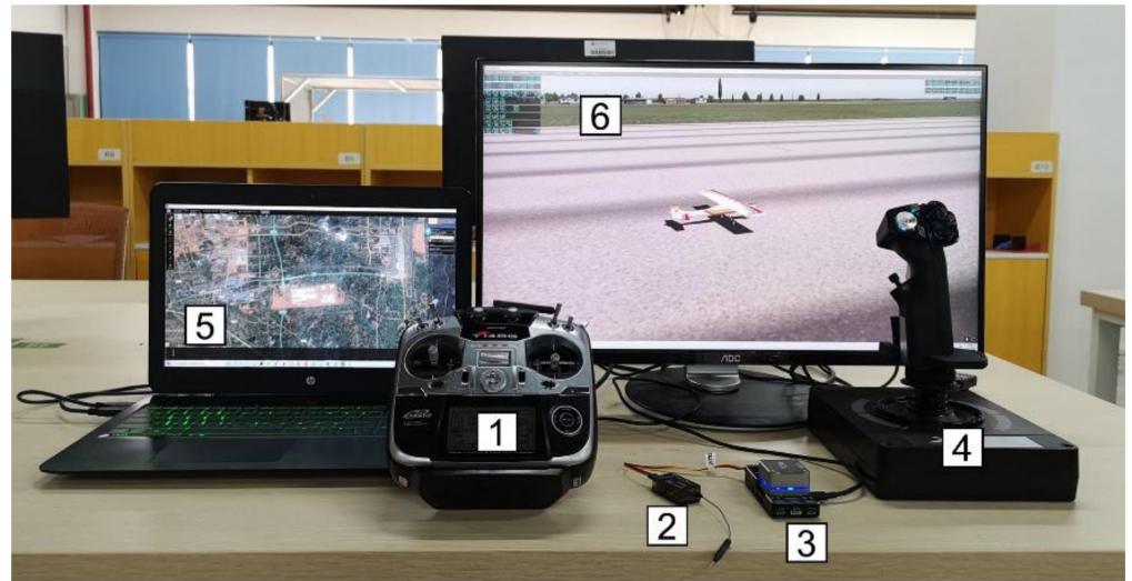
Figure 3. Flight maneuver demonstration and learning system including (1) remote controller, (2) signal receiver, (3) Pixhawk-v5, (4) flight joystick, (5) ground control station, and (6) flight simulation software X-Plane.
