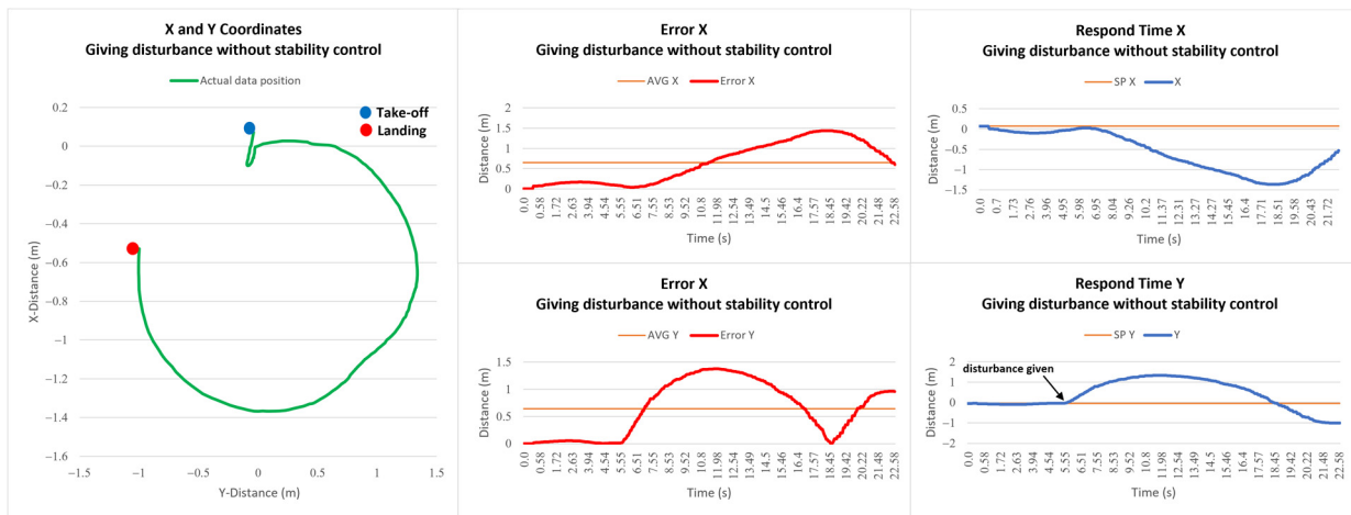
Figure 11. The response result from adding disturbance during hovering without stability mode control.
