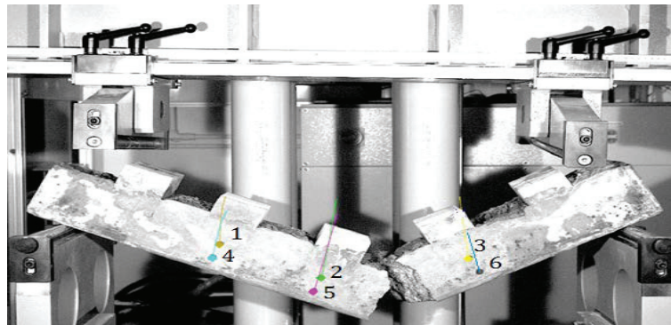
Figure 14. Sample after bending strength testing—dots were used to register the movement of the sample with the PHANTOM MICRO LC310 camera—not described in this article.
