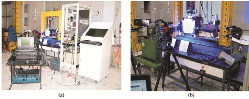
Figure 5. View of the test stand in operation: (a) overall view, (b) specimen view; 1—the test stand with the fixed actuators; 2—a test element; 3—the hydraulic system ‘A’; 4—the hydraulic system ‘B’; 5—the measurement and control interface; 6—IT system; 7—cameras of the ARAMIS 6M system; 8—PUNDIT LAB+ instrument.
