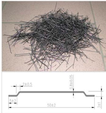
Figure 3. Fibre dimensions and close-up look.
