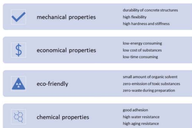
Figure 3. Critical aspects in the field of challenges of production of coating materials used for protection of concrete elements.
