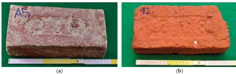
Figure 2. (a) historical solid brick—high firing temperature, (b) historical full brick—low firing temperature.
