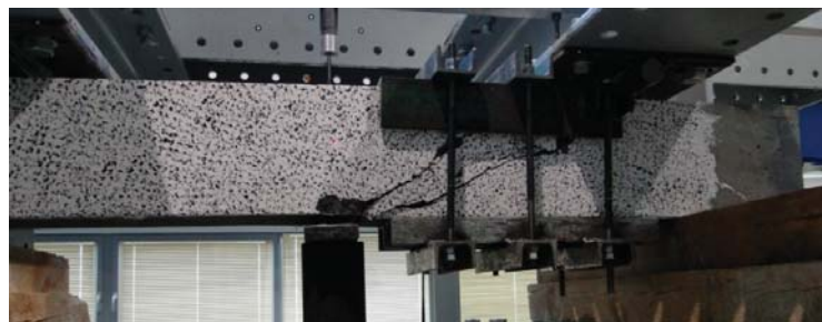
Figure 8. Beam reinforced with steel corset after the first testing stage.
