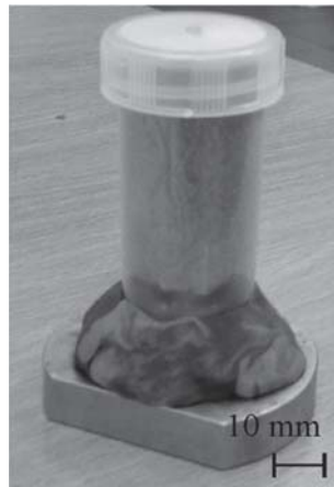
Figure 1. A medium sand sample prepared for testing in microtomography.
