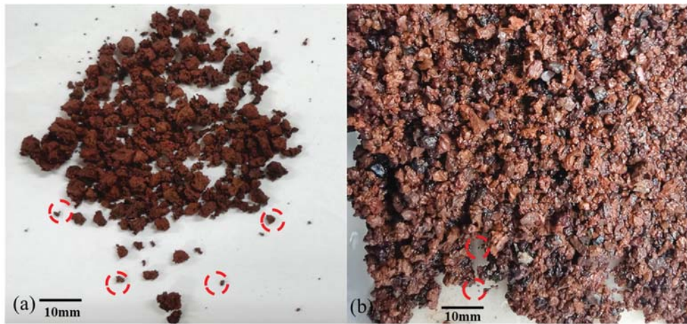
Figure 19. Photos of volcanic soil after shear test: (a) 2–5 mm-0.7–400 kPa test sample; (b) 0.5–2 mm-0.7–400 kPa test sample.
