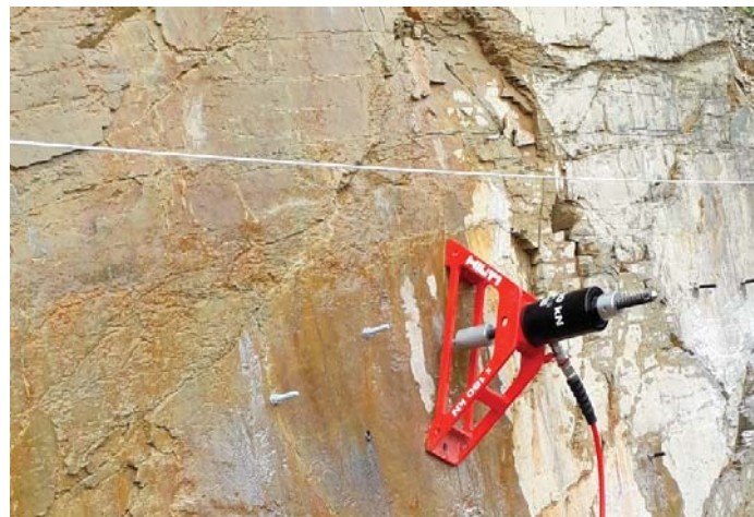
Figure 1. Test setup with hydraulic handpump, wide load bridge and scanline.
