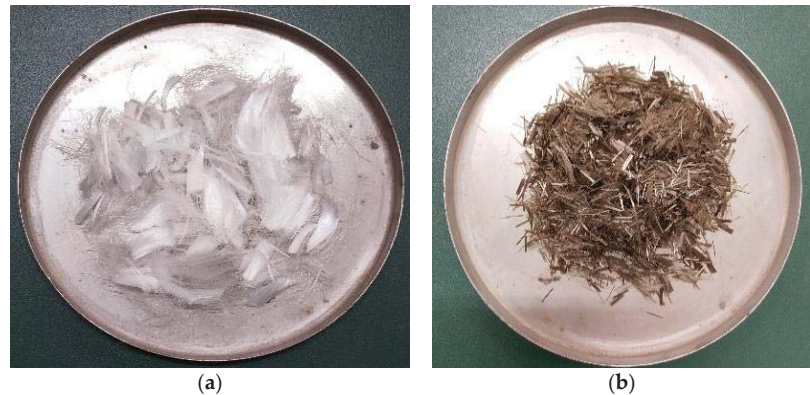
Figure 1. The appearance of fiber. (a) Polypropylene fiber and (b) basalt fiber.
