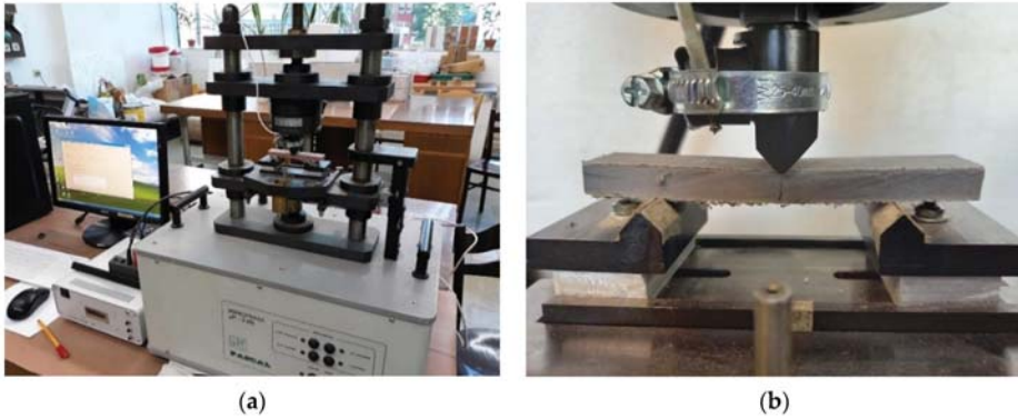
Figure 5. Test stand for acoustic emission measurements and the fibre cement board used during the test: (a) view of the testing machine; (b) view of the specimen during its destruction.
