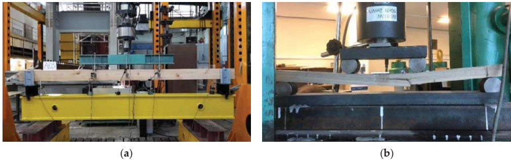
Figure 4. View of experimental stands for testing: (a) technical scale beam, (b) small clear specimen (Group 2).
