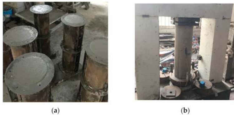
Figure 5. Unreinforced specimens. (a) Specimens pouring; (b) Completed specimen.
