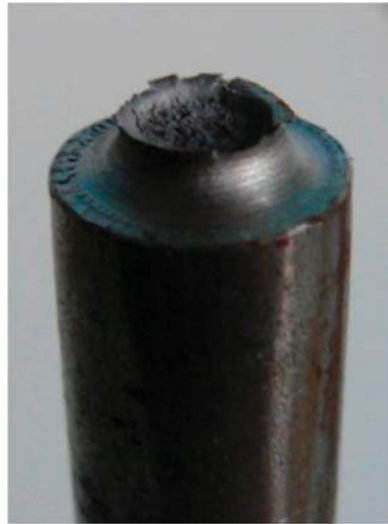
Figure 11. Macroscopic photograph of a fracture surface of a tensile notched specimen. Transition from the flat failure mechanism in the specimen center to the slant fracture at the edges is clearly visible. The first mechanism involves normal stress, while in the latter, shear stress plays a dominant role.
