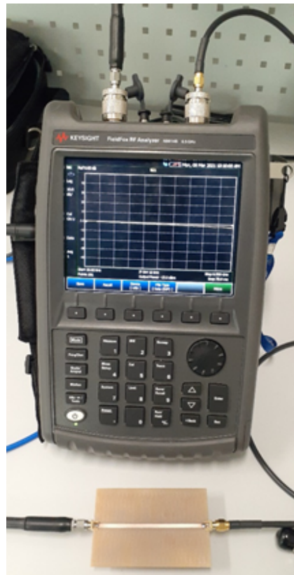
Figure 8. Measurement Setup for Transmission Loss.
