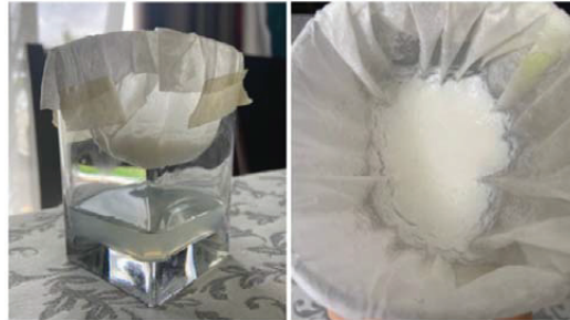
Figure 7. Filtration of casein precipitated from a sample of milk (Images extracted from a students' report).
