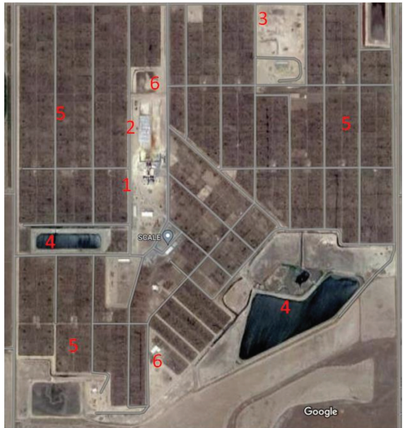
Figure 4. Aerial image of randomly chosen commercial feedyard. Feedmill is indicated by 1; silage pits are depicted by 2; manure/pen surface composting is tagged 3; 4 denotes water retention pond; 5 indicates cattle pens; and 6 highlights cattle working facilities. Image selected from Google Maps.
