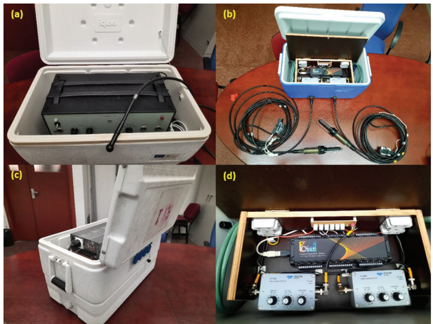
Figure 5. Images of the HW platform implementation: (a) transmitter unit, (b) receiver unit for 2 hydrophones, (c) power inverter unit and (d) top view of the receiver unit.
