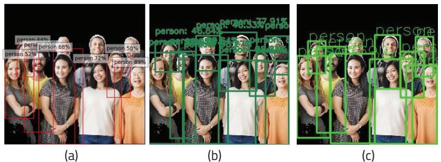
Figure 24. Results for different frameworks: (a) SSD, (b) MobileNet, and (c) Faster R-CNN.
