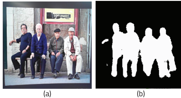
Figure 7. Results of masking: (a) original frame and (b) masked image.
