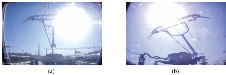
Figure 11. Sun affects pantograph detection. (a) HSR-A. (b) HSR-B.
