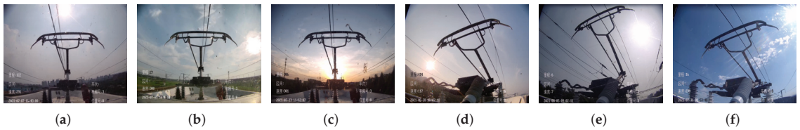
Figure 16. Sun did not affect YOLO detection of pantographs in HSR-A and HSR-B. (a) Case I. (b) Case II. (c) Case III. (d) Case IV. (e) Case V. (f) Case VI.
