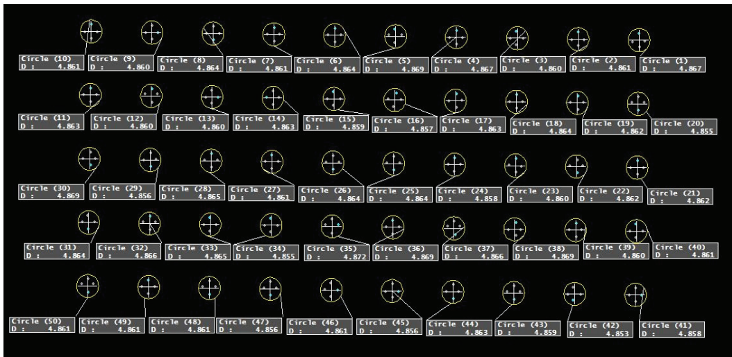
Figure 6. Example of hole diameter measurement for AL7075-T6 panel.
