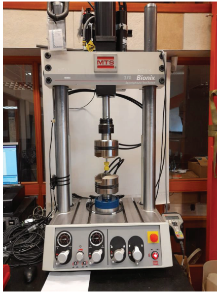
Figure 5. MTS858 Bionix fatigue test stand used for PUR fatigue testing.
