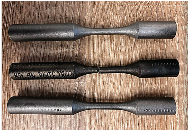
Figure 4. Photograph of test specimens before and after axial fatigue testing, OUtech Opole.
