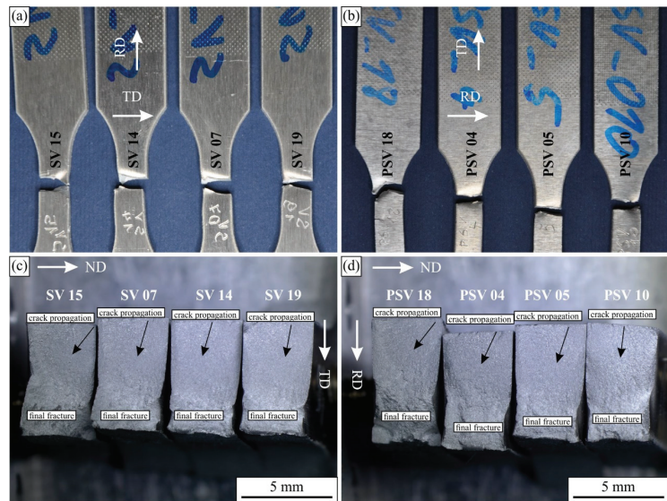
Figure 9. The light micrographs of the fractured surfaces of the selected fatigue samples: (a,c) longitudinal layout and (b,d) transverse layout (ND—normal direction, RD—rolling direction, TD—transverse direction).
