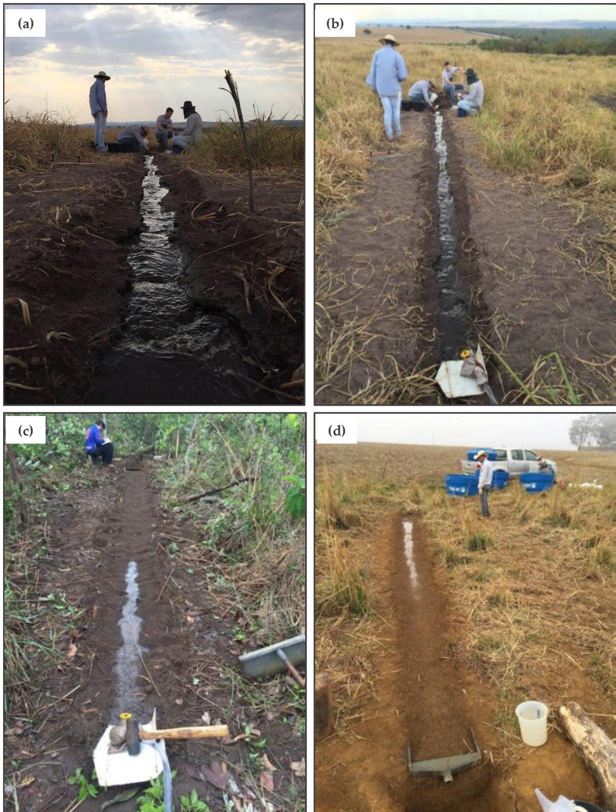
Figure 2. Preparation of areas for determination of erodibility in the furrow (Kr): (a,b) in the watershed under pasture, (c) in the micro-basin under native vegetation, and (d) in the micro-basin under agriculture.
