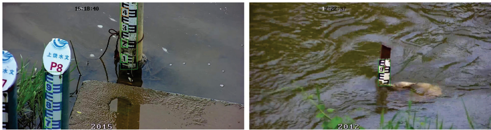
Figure 10. Dirty water gauge image inspection results.
