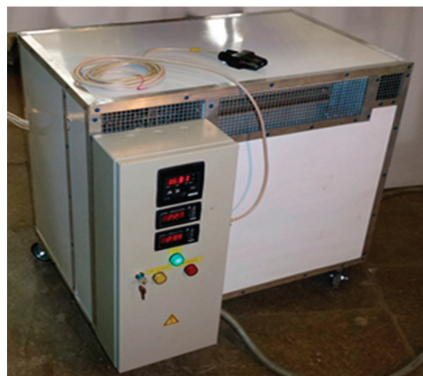
Figure 2. Electric thermal storage unit.
