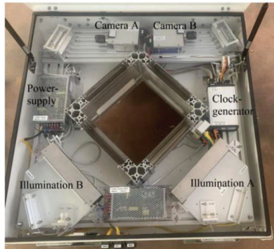
Figure 4. 2DVD system used to measure the characteristics of rainfall drops.
