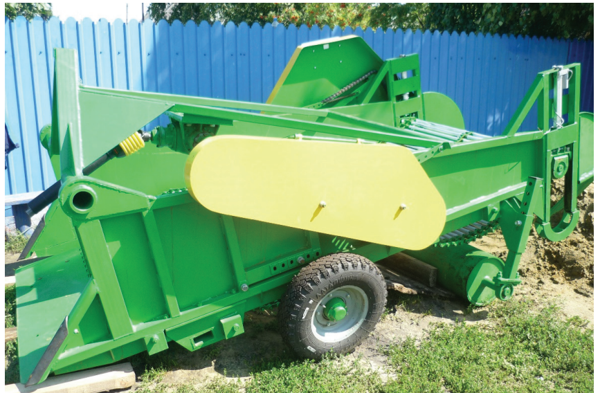
Figure 5. General view of the harvesting machine for root crops and onions, equipped with a separating rod elevator with an adjustable blade inclination angle and a receiving plowshare for digging/picking up root crops and bulbs.
