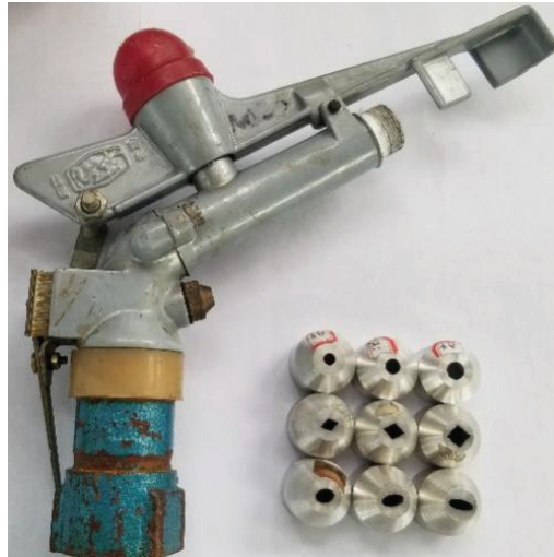
Figure 3. Photograph of the sprinkler and nozzles used in experiments.
