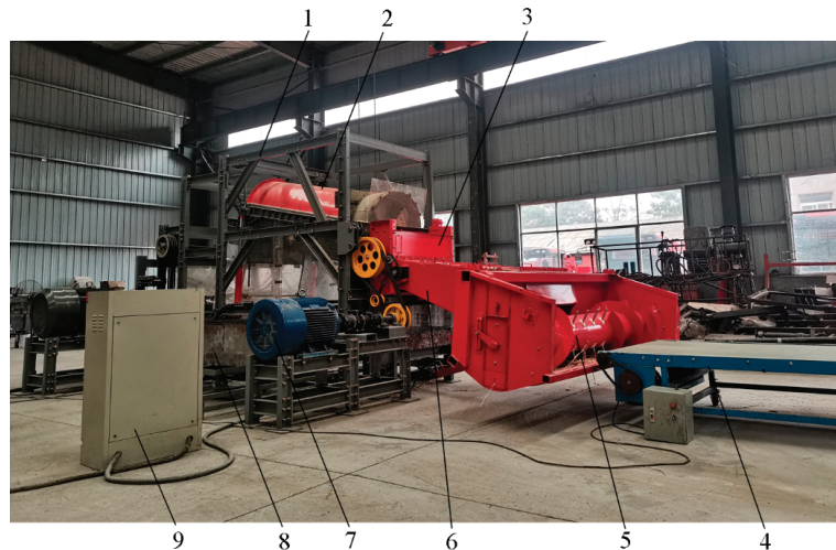
Figure 3. Structural view of the threshing test bench. 1. Frame; 2. Longitudinal axial flow threshing and separating device; 3. Tangential flow threshing and separating device; 4. Material conveying platform; 5. Inclined conveyor; 6. Screw conveyor; 7. Motor; 8. Grain collection boxes; 9. Frequency converter.
