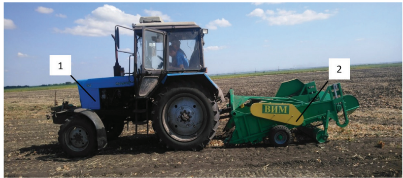
Figure 6. General view of the harvesting unit for harvesting root crops and onions, equipped with a separating rod elevator with an adjustable blade inclination angle: 1—MTZ 1221 tractor; and 2—machine for harvesting root crops and onions.
