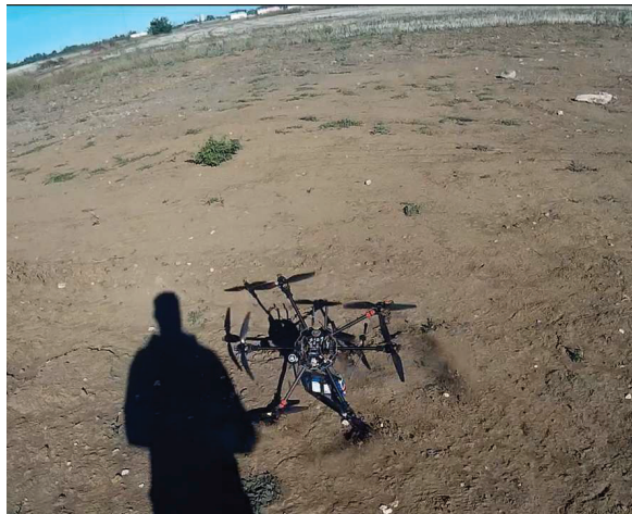
Figure 44. Hexacopter impact during field tests.
