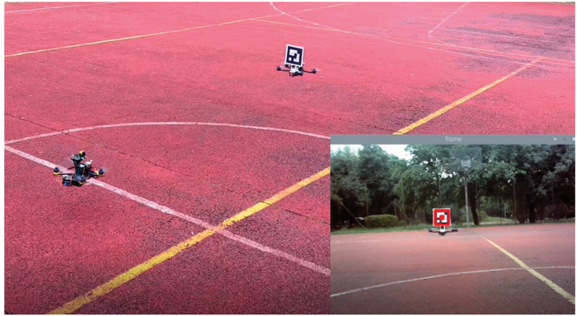
Figure 8. Flight in a straight line behind the leader. The bottom right image was taken by the camera, showing the detected marker.
