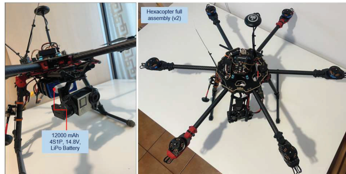
Figure 5. Hexacopter assembly for variant v2.
