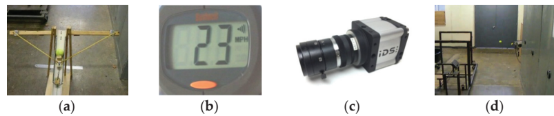
Figure 4. Real world experimental setup. (a) Ball throwing device. (b) Radar gun to measure launching speed. (c) Used camera (UI-1220RE-M-GL). (d) Trajectory captured through throw side camera.
