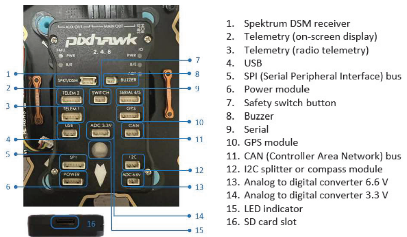
Figure 9. Pixhawk 2.4.8 flight controller and the peripheral connection interfaces.
