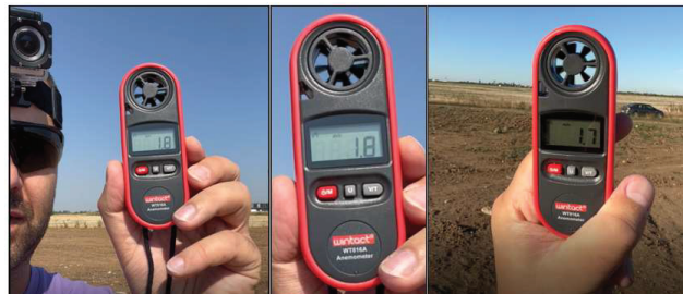
Figure 23. Wind speed measurement with anemometer.
